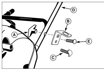
Figure 7. Mounting Lower Bracket (520) A. Wing Lock Knob D. Handle, LH
